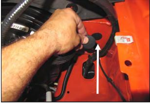
**5.** Plug the resonator hole in the firewall with the Firewall Plug (#15).
