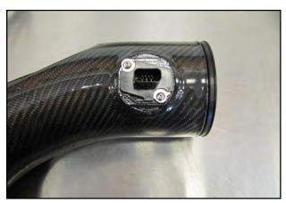
**8.** Install the Mass Air Flow sensor into the intake tube using two provided 8-32x3/8" screws (#11).
