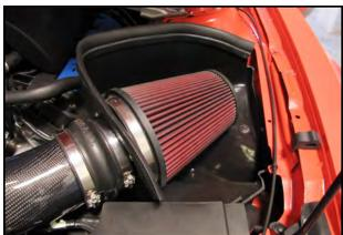
**15.** Install the Airaid Premium Filter (#1) onto the filter adapter and tighten the hose clamp.
