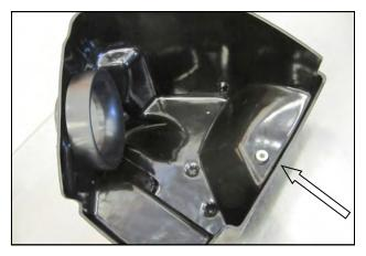
**10.** Remove the factory upper air box mounting grommet and steel sleeve, and re-install into the Airaid **CAB**.
