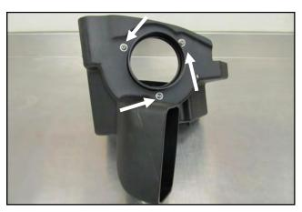
9. Install the Filter Adapter (#7) onto the Airaid Cool Air Box (#4) as shown.
