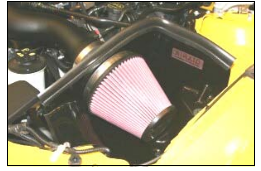
15. Install the Airaid Premium Filter (#1) onto the filter adapter (#5). Next install the weather strip (#7) on the top of the CAD as shown. Start at the front of the CAD and work towards the rear.
