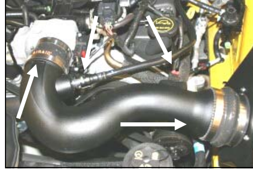
14. Install the Airaid Intake Tube into the hump hose first, and then into the reducing coupler, adjust for fit, and then tighten the four hose clamps. Reconnect the breather hose, and the wiring harness to the MAF sensor.
