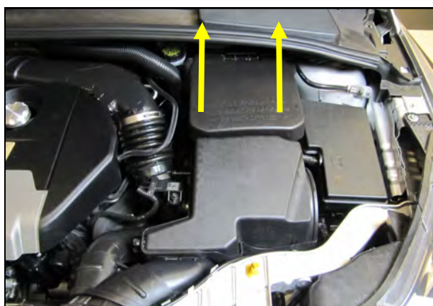
2. Locate battery cover and remove it. Disconnect the Negative terminal.
