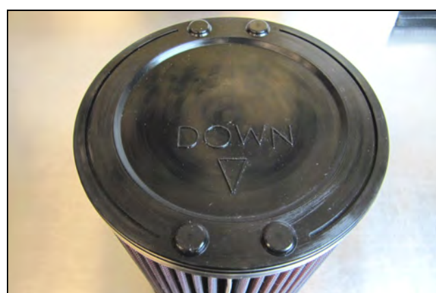
6. Notice that the Airaid Filter top has a directional arrow in the center and locating lugs in the 12:00 and 6:00 positions.
