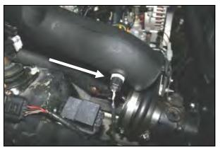
11. Carefully install the factory intake temp sensor (if equipped) into the grommet in the Airaid Intake Tube. Skip this step if your vehicle doesn't have an intake temp sensor.
