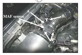
2. A.) Loosen the factory intake tube hose clamp on the Mass Air Flow (MAF) sensor housing. B.) Carefully remove the intake air temperature sensor (if equipped) from the factory intake tube. C.) Using the supplied T-20 torx bit, remove two screws, and remove the MAF sensor from the MAF housing. Set the temp sensor and MAF sensor to the side for reinstallation later.
