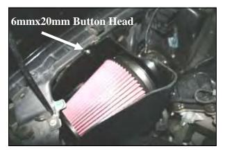
9. Install the Airaid Premium Filter (#1) onto the velocity stack inside of the **CAD** as shown and tighten the clamp. Next install the **CAD** assembly into the vehicle aligning the grommet posts into the factory grommets in the inner fender. Now secure the **CAD** to the inner fender well using the 6mmx20mm button head bolt (#9), and flat washer (#11).
