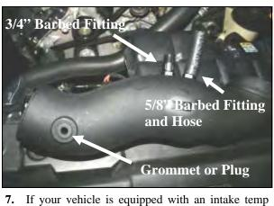
sensor, install the supplied grommet (#17) into the hole in the Airaid Intake Tube (#2), if not, install the grommet plug (#18). Next install the two barbed fittings (#19 & #20) into the tube as shown. Now install the 5/8"x 3" hose (#16) onto the 5/8" barbed fitting.
