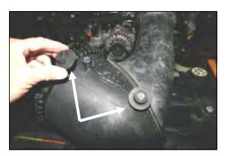
**4.** Remove the two factory grommets from the bottom of the factory air filter canister and reinstall them into the holes in the inner fender.
