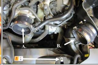
11. Install the Coupler and Hump Hose and Clamps: tle body side of the reducer, and the #64 clamp (#18) on your application. Leave the Clamps loose for now.
