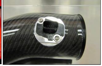
5. Insert the Fire Wall Plug (#16) into the resonator hole. 6. Using the supplied Torx bit, (#19) remove the MAF sensor from the factory airbox and transfer it into the Airaid Tube assembly (#2).
