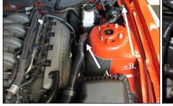
4. Remove the resonator assembly from the vehicle. A. Slide the hanger off of the strut tower tab.
