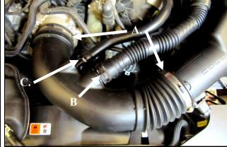
2. A) Loosen the hose clamps on the factory intake tube B) Squeeze the spring clamp and disconnect the resonator from the air intake tube. C) Carefully depress the hose lock tab, and disconnect the crank case breather line and the brake aspirator line if equipped, (AT models only). D) Remove the factory intake tube.
