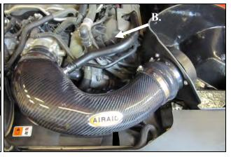
12. Install the Airaid Intake Tube into the couplers as A. Install the Silicone Coupler (#6) and Hose clamps onto shown, and tighten all Hose clamps. Reconnect the the throttle body. Place the #56 clamp (#15) on the Throt- breather line/lines to the Aluminum Fittings depending on
