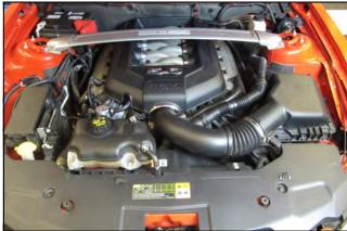
**Disconnect The Negative Battery Terminal!** 1. If so equipped, remove the strut tower brace, then remove the engine cover by simply lifting it up, and set aside.
