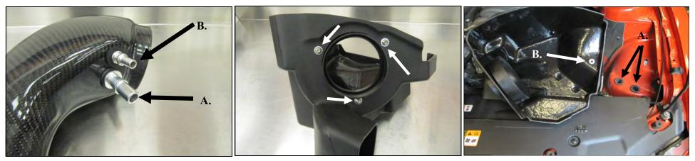
7. Install the Grommets and Fittings into the Airaid Intake 8. Install the filter adapter (#4) using three 1/4-20 button Tube (#2): A) All models will require the use of the 5/8" Fitting (#15) and the 5/8"Grommet (#12). B) Automatic transmission equipped vehicles will also use the 3/8" Fitting (#14) and 3/8" Grommet (#11). Manual transmission vehicles will not need the 3/8" components and will use the Blind Grommet(#13
