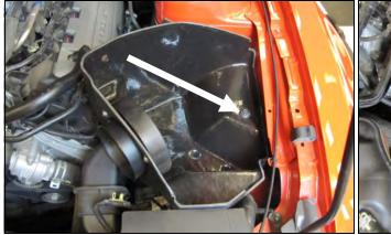
10. Install the CAB into the vehicle. Make sure that the Air inlet of the CAB aligns with the factory duct, and the two locating pins on the bottom align with the factory grommets. Next reinstall the factory bolt that was removed in step #3 through the steel sleeve and grommet and into the inner fender.
