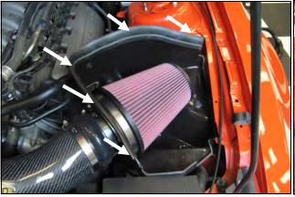
13. Install the Airaid Premium Filter (#1) onto the Flter Adapter and tighten the hose clamp. Install the Weather Strip (#7) onto the CAB with the contoured edge going away from the filter. Start at the front of the vehicle and work your way back.
