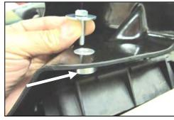
**9.** Slide the Aluminum Spacer (#14) underneath the **CAD** and into the hole as shown. Secure the CAD to the inner fender using the OEM bolt from step #3 and the supplied 1/4" Fender Washer (#15).
