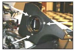
7. Install the air filter adapter (#5) into the Cool Air Dam (#7) as shown, using 3 button head bolts (#9) and ½" flat washers (#10).
