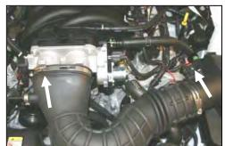
**2.** Loosen the intake tube hose clamp on the throttle body. Slide the red tab on the electrical connector, and disconnect the mass air sensor.
