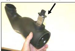
12. Align the two slots in the tubes, and install the factory mass air sensor removed from step #5. Make sure the screw holes line up, then install the two supplied button head screws. (#11). DO NOT USE THE FACTORY SCREWS!!
