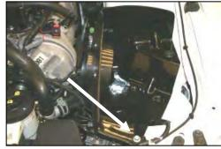
8. Place the CAD into the inner fender, align the bolt holes and re-install the bolt from step
