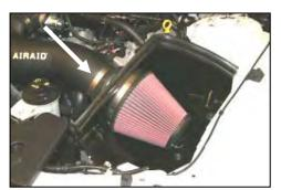
**15.** Install the Airaid Premium Filter (#1) onto the filter adapter, and tighten the clamp. Install the weather strip (#8) on the top of the **CAD** as shown
