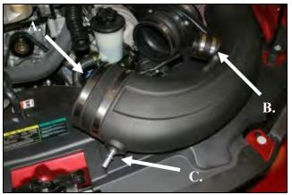
now. B.) Install the 1 3/4" coupler (#6) onto the intake tube using two #28 hose clamps (#16) as shown. Tighten only the clamp against the tube for now. C.) Install the provided grommet (#17) into the intake tube and then install the aluminum fitting (#20) into the grommet as shown.
