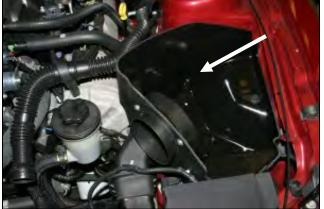
scoop, and the two locating pins on the bottom align with the factory grommets. Next reinstall the factory bolt that was removed in step #2 thru the steel sleeve and grommet and into the inner fender. Make sure that the wiring harness is not pinched under the CAB.
