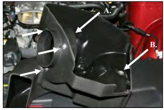
button head bolts (#11), and flat washers (#10) into the as shown. Now reinstall the wiring loom anchors into scoop provision in the CAB aligns with the factory Airaid Cool Air Box (CAB) (#3) as shown. B.) Reinstall their respective holes starting at the back of the CAB the small grommet and sleeve (removed in step #3) into with the two hole anchor and work your way underneath the hole in the CAD.
