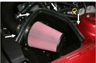
adapter and tighten the hose clamp. Next, install the connectors, cut the factory breather tube on each end just weatherstrip (#9) onto the top of the CAD as shown start- enough to remove the factory connectors. ing near the radiator and working your way towards the left fender.
