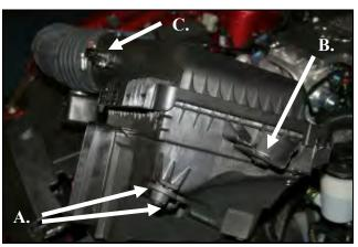
3. Grab the airbox and tube and roll it forward while lifting up to dislodge it from the intake scoop. Remove the assembly from the vehicle. A.) Remove the two factory grommets and then replace them back into the two holes in the inner fender. B.) Remove the steel sleeve and grommet and save for reinstallation later. C.) Using the provided #20 Torx bit, remove the two screws and the **MAF** sensor from the tube.
