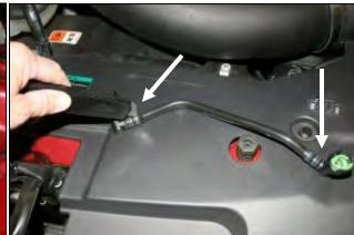
14. Install the Airaid Premium Filter (#1) onto the filter 15. VERY CAREFULLY! Without cutting thru the
