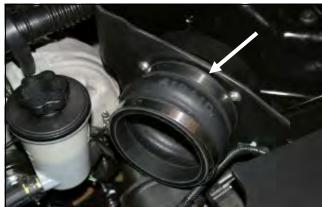
7. Install the provided hump hose (#4) onto the filter 8. Install the MAF sensor into the intake tube using two adapter using two #72 hose clamps (#15) as shown. Leave the two hose clamps loose for now.
