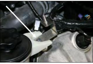
11. Install the bracket assembly from step #10 as shown. 12.A.) Install the oval coupler onto the intake tube using This bracket and 6mm bolt will secure the power steering two #72 hose clamps (#15). Leave the clamps loose for reservoir and replaces the stud removed in step #9.
