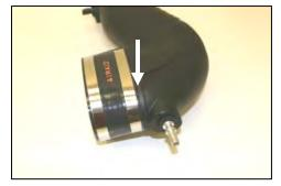
**14.** Install the oval coupler (#4) with two #72 hose clamps (#13). Tighten only the clamp closest to the aluminum fitting. (*Hint: For a clean look, locate the hose clamp tightening screws under the tube*)!
