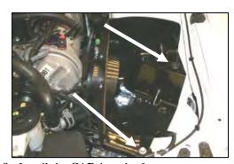
**9.** Install the **CAD** into the factory grommets in the inner fender, and re-install the bolts from steps #3 and #6.
