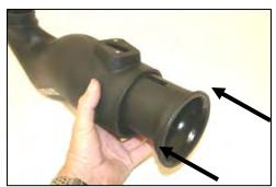
12. Install the Modular Venturi Tube (MVT) (#3) into the Airaid Intake Tube (#2) as shown. (SEE #22 BELOW!!)
