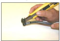
**17.** <u>VERY CAREFULLY !</u> Using a razor blade, cut the plastic tube off both of the factory breather hose ends as shown.
