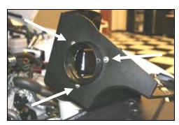
**8.** Install the air filter adapter (#6) into the Cool **Air D**am (#7) as shown, using 3 button head bolts (#10) and <sup>1</sup>/<sub>4</sub>" flat washers (#11).
