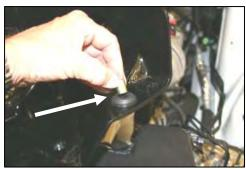
7. Install the provided grommet (#15), with the groove at the top, into the Cool Air Dam (CAD) hole, as shown. Next slide the aluminum sleeve (#16), into the center of the grommet.
