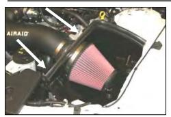
**16.** Install the Airaid Premium Filter (#1) onto the filter adapter, and tighten the clamp. Install the weather strip (#9) on the top of the **CAD** as shown.
