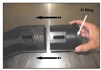
7. Slide the Modular Venturi Tube (#3) into the Airaid Intake tube (#2). Make sure to align the two slots for the Mass Air Flow sensor and that the O Ring (#18) is in Place.
