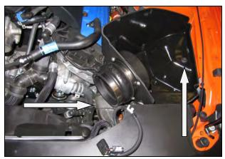
12. Install the CAD into the vehicle. Make sure that the air inlet of the CAD aligns with the factory duct, and the two locating pins on the bottom are seated in the factory grommets. Next reinstall the factory bolt that was removed in step #3 thru the steel sleeve and grommet and into the inner fender.
