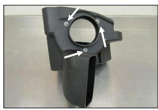
9. Install the Filter Adapter (#7) onto the Airaid Cool Air Box or (CAB) (#4) as shown.
