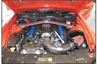
16. Reconnect the Mass Air Flow sensor, which is now located in the lower back side of the intake. Slide the locking tab back into the connector.
