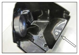
10. Remove the factory upper air box mounting grommet and steel sleeve, and re-install into the Airaid CAD.
