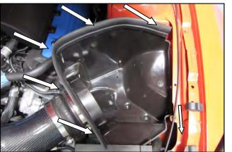
14. Install the Weather Strip (#8) onto the CAD with the contoured edge rolling away from the filter area. Start at the front of the vehicle and work your way back
