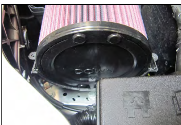
7. Install The Airaid Premium Filter (#1) and clamp into the air box as shown with the Arrow pointing Down and the Lugs in the correct position. When properly installed, the Filter top will be completely inside of the airbox, lower half.
