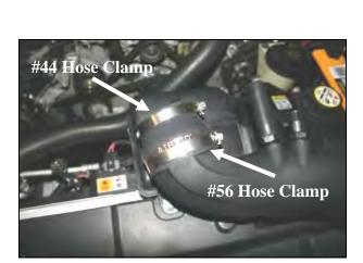
**8.** Install the reducer coupler (#4) onto the throttle-body end of the Airaid Intake Tube using the #56 hose clamp (#14) on the tube end, and the #44 hose clamp (#13) on the small end. Tighten *only* the large #56 clamp at this time.
