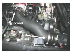
**12.** Install the Airaid Intake Tube into the hump hose first, and then onto the throttlebody. Adjust for fit, and then tighten the two remaining hose clamps. Reconnect the crankcase breather hose to the 5/8"x 3" hose, and connect the idle bypass hose to the 3/4" barbed fitting. Now reinstall the **MAF** sensor onto the **MAF** housing using the factory screws.
