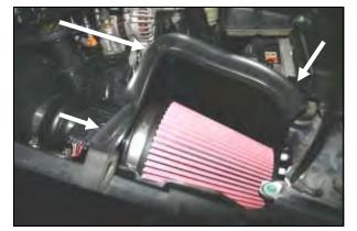
**13.** Install the supplied weather strip (#7) onto the top of the **CAD** starting at the fender and working your way towards the radiator.
