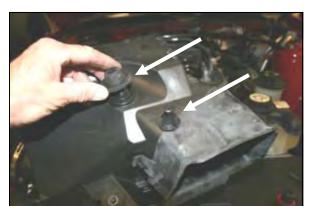
**4.** Remove the two factory grommets from the bottom of the factory airbox and replace them back into the holes in the inner fender. They will be used to guide the Airaid Cool Air Dam to the correct location in the vehicle.
