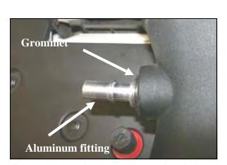
7. Install the provided grommet (#11) into the large hole in the side of the Airaid Intake Tube (#2). Next, carefully install the supplied aluminum fitting (#14) into the grommet as shown.
