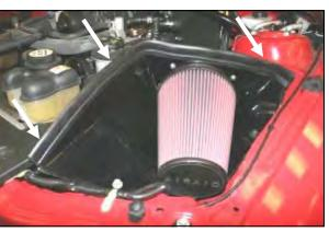
**14.** Install the Airaid Premium Filter (#1) onto the Airaid Intake Tube and tighten the hose clamp. Next install the supplied weather strip (#5) onto the top of the **CAD** as shown. For ease of installation, start next to the radiator and work your way towards the fender.
