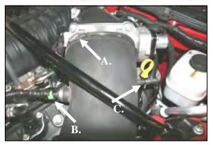
**2.** A.) Loosen the factory intake tube hose clamp on the throttle body. B.) Push the GREEN tab on the breather hose connector and disconnect it from the factory intake tube. C.) CAREFULLY disconnect the vacuum line from the factory intake tube.
