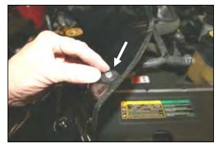
**12.** Install the tall grommet (#12) with the groove at the top, into the hole in the Cool Air Dam (#3). Next push the supplied aluminum sleeve (#10) into the hole in the grommet as shown.
