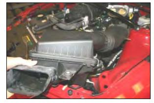
**3.** Remove the complete factory intake system from the vehicle.
