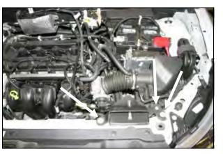
1. Disconnect the negative battery cable! Remove the three bolts that secure the intake scoop to the radiator support. The two long bolts will be reused in step #14.
