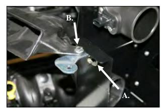
**13. A.**) Install the front bracket (#18) onto the front of the **CAD** as shown using one 1/4"-20x5/8" hex bolt (#13), two 1/4" flat washers (#12), and one lock nut (#14). **B.**) Next mount the factory scoop to the bracket as shown using one 1/4"-20x5/8" hex bolt (#13), two 1/4" flat washers (#12), and one lock nut (#14).
