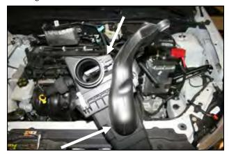
5. Remove the scoop from the factory airbox. Next, usinstalled in steps #10 & 13.
