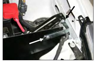
**15.** Install the side bracket (#17) onto the **CAD** as shown using the factory bolt removed in step #6, and one 1/4"-20x5/16 hex bolt (#13), two 1/4" flat washers (#12), and one lock nut (#14).
