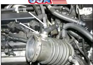
**3.** Remove the factory flexible intake tube from the vehicle. Remove the Oeticker clamp, and then remove the large plastic elbow from the flexible intake tube. It will be reused in step #12.
