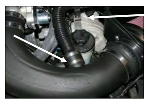
**1.** Loosen the clamps on the resonator tube coupler and disconnect it from the intake tube. Pull up on the resonator tube to release it from the resonator
