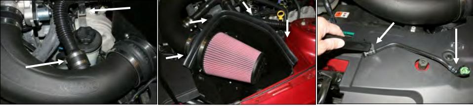
and then onto the throttlebody. Adjust for fit and then tighten all four hose clamps. Next, reinstall the factory resonator tube into the 1 3/4" coupler and tighten the hose clamp. Now "reseat" the resonator tube onto the bracket.
