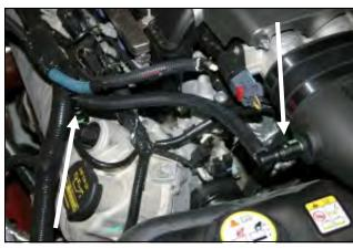
16. Install the two factory connectors from step #15 into each end of the supplied 3/8"x12" breather hose (#10). Now reattach one connector to the valve cover, and the other end to the aluminum fitting on the intake tube.
