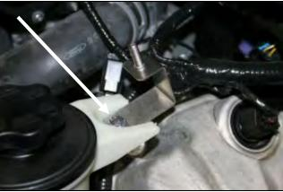
**11.** Install the bracket assembly from step #10 as shown. 12.A.) Install the oval coupler onto the intake tube using This bracket and 6mm bolt will secure the power steering two #72 hose clamps (#17). Leave the clamps loose for reservoir and replaces the stud removed in step #9.
