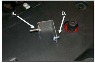
10.A.) Thread the 1/4-20 hex bolt (#15) into the resonator bracket (#22) and tighten as shown. **B.**) Slide the 6mmx12mm (#16) hex bolt thru one flat
