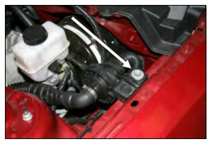
**5.** Remove the bolt that secures the resonator tube and diaphragm to the left inner fender.
