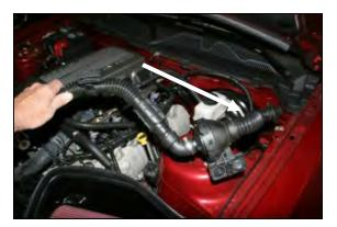
**6.** Grab the resonator tube between the diaphragm and the firewall and pull up and out to disconnect it from the firewall. Remove the complete resonator assembly from the vehicle.
