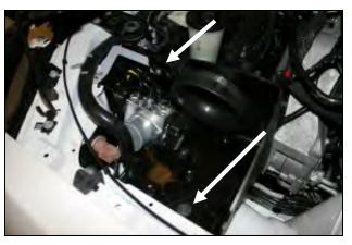
**9.** Install the **CAD** into the vehicle aligning the locating pins on the bottom of the **CAD** into the factory grommets in the fender. Reinstall the factory bolt from step #2 into the steel sleeve and grommet. Next install the 1/4-20x5/8" hex bolt (#14) thru one 1/4" flat washer (#9), thru the **CAD**, and thru the bracket securing it with one 1/4" serrated nut (#15). Adjust for fit and then tighten the bolt on the anti lock brake bracket.
