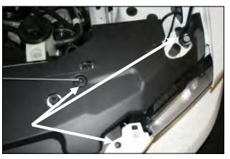
**6.** Using a flat blade screwdriver, pry up the center of the three plastic trim anchors that are shown. Once the center is up, then pry up the bottom half of the anchors up and out of the hole and save them for reinstallation in step #10.
