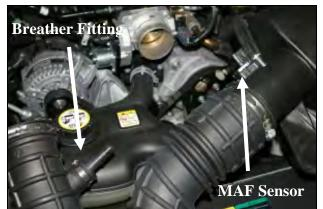
**5.** Using the supplied #20 torx bit, remove 2 factory screws, and remove the **MAF** sensor from the factory tube. (Save the **MAF** sensor for reinstallation in step #12). Next, using a pair of side cutters, remove the metal band that holds the plastic breather fitting into the factory back and the facto
