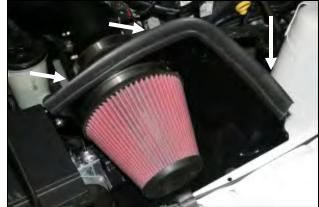
**14.** Install the Airaid Premium Filter (#1) onto the filter adapter as shown and tighten the clamp. Now install the supplied weather strip (#7) onto the top of the **CAD** as shown starting near the radiator and working towards the left fender.
