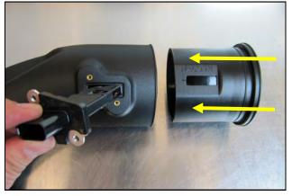
tube using two provided 8-32x3/8" screws (#12).
