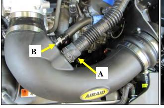
11. Install the Airaid Intake Tube into the couplers as 12. A) Install the Airaid Premium Filter onto the filter shown, and tighten all Hose Clamps. A) Reconnect the adapter and tighten the hose clamp. B) re install the Reso-Resonator tube to the Airaid Intake using the OEM nator tubing into the factory Stand off. clamp. B) Reconnect the breather line/lines to the Aluminum Fittings depending on your application.
