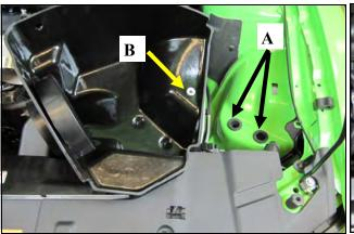
7. Transfer the factory air box mounting grommets. A) Locate and remove the Two Lower air box mounting grommets, and install them in the inner fender. B) Remove the Upper air box mounting grommet and steel sleeve, and re-install into the Airaid Cool Air Box
