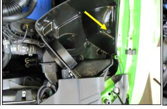
**8.** Install the Cool Air Box into the vehicle. Make sure that the Air inlet mates with the factory duct, and the two locating pins on the bottom align with the factory grommets. Next reinstall the factory bolt that was removed in step #3 through the steel sleeve and grommet and into the inner fender.
