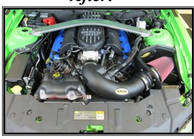
Synthamax Air Filters do not require oil. Service air filter as needed by cleaning with common non-petroleum all-purpose household cleaner and water. Simple Green®, Formula 409® or equivalent works great. Apply cleaner to outside of air filter and allow to soak. Then flush filter clean from the inside out with a garden hose and repeat steps if necessary. Do not apply high pressure water or air to clean filter. Allow filter to air dry and reinstall.
