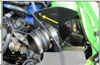
9. Install the hump hose onto the filter adapter using two #72 hose clamps (#13) as shown. Leave the two hose clamps loose for now. Transfer the Resonator stand off from the factory air box into the Cool Air Box.
