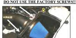
16. Install the Airaid Premium Filter (#1) onto the filter adapter, and tighten the clamp. Install the weather strip (#9) on the top of the CAD as
