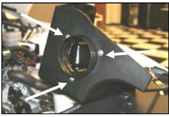
7. Install the air filter adapter (#5) into the Cool Air Dam (#7) as shown, using 3 button head bolts (#9) and ½" flat washers (#10).
