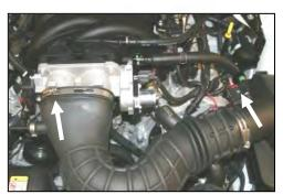
**2.** Loosen the intake tube hose clamp on the throttle body. Slide the red tab on the electrical connector, and disconnect the mass air sensor.
