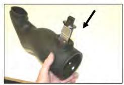
13. Align the two slots in the tubes, and install the factory mass air sensor removed from step #5. Make sure the screw holes line up, then install the two supplied button head screws. (#13).
