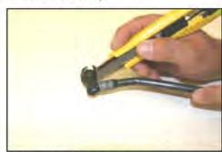
17. VERY CAREFULLY! Using a razor blade, cut the plastic tube off both of the factory breather hose ends as shown.
