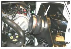
**10.** Install the hump hose (#5) on the filter adapter (#6), with two #72 hose clamps (#13). Tighten only the clamp next to the **CAD**.
