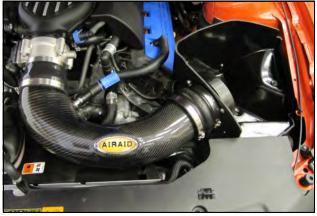
**13.** Install the Airaid Intake tube onto the throttlebody first then into the Hump Hose and tighten the clamps. Reconnect the crank case breather line to the Aluminum fitting on the Intake Tube.
