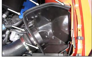
**14.** Install the Weather Strip (#8) onto the **CAB** with the contoured edge rolling away from the filter area. Start at the front of the vehicle and work your way back
