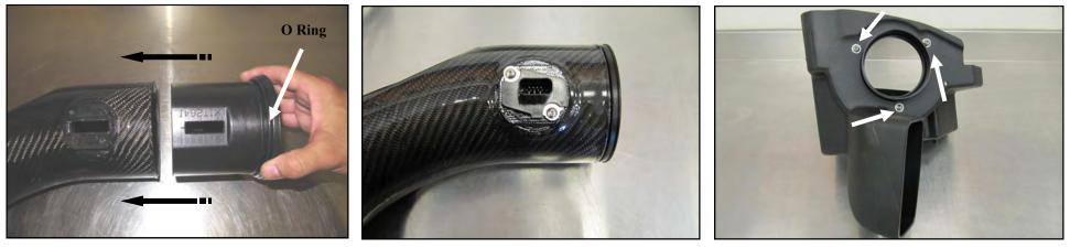
**7.** Slide the Modular Venturi Tube (#3) into the Airaid Intake tube (#2). Make sure to align the two slots for the Mass Air Flow sensor and that the O Ring (#18) is in Place.
