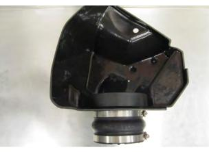
**11.** Install the hump hose (#5) and two #72 hose clamps (#12) onto the filter adapter as shown. Leave the two hose clamps loose for now.
