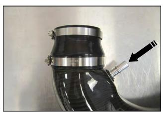
**6. A.)** Install the Silicone Reducer (#6) and Hose clamps onto the Airaid Intake Tube (#2). Place the #56 clamp (#14) on the Throttle body side of the reducer, and the
