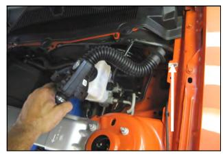
**4.** Unbolt the Intake resonator from the inner fender and disconnect it at the drivers side firewall. Remove the entire assembly from the vehicle and set it aside. It will
