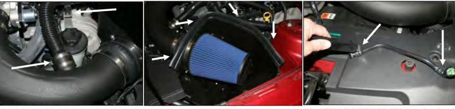
and then onto the throttlebody. Adjust for fit and then tighten all four hose clamps. Next, reinstall the factory resonator tube into the 1 3/4" coupler and tighten the hose clamp. Now "reseat" the resonator tube onto the bracket.
