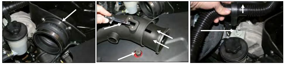
7. Install the provided hump hose (#5) onto the filter 8. Slide the Modular Venturi Tube (#3) into the Airaid adapter using two #72 hose clamps (#17) as shown. Leave the two hose clamps loose for now.
