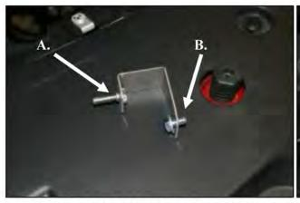
10.A.) Thread the 1/4-20 hex bolt (#15) into the resonator bracket (#22) and tighten as shown.
