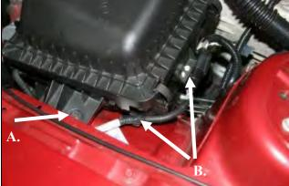
2.A.) Using a 10mm socket, remove and save the bolt that secures the airbox to the fender.
