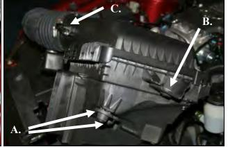
3. Grab the airbox and tube and roll it forward while lifting up to dislodge it from the intake scoop. Remove the assembly from the vehicle. A.) Remove the two factory grommets and then replace them back into the two holes in the inner fender. B.) Remove the steel sleeve and grommet and save for reinstallation later. C.) Using the provided #20 Torx bit, remove the two screws and the MAF sensor from the tube.
