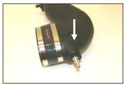
**13.** Install the oval coupler (#3) with two #72 hose clamps (#12). Tighten only the clamp closest to the aluminum fitting. (*Hint: For a clean look, locate the hose clamp tightening screws under the tube*)!
