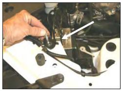
**6.** With a 10mm socket, remove and save the bolt from the anti-lock brake bracket. It will be re-installed later in step #9.
