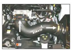
**14.** A.) Install the tube into the hump hose. B.) Now slide the oval coupler onto the throttle body. Tighten the remaining two hose clamps, and re-connect the mass air sensor, from step #2.
