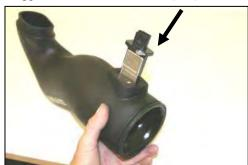
the factory mass air sensor removed from step #5. Make sure the screw holes line up, then install the two supplied button head screws. (#11). DO NOT USE THE FACTORY SCREWS!!
