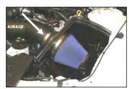
**15.** Install the Airaid Premium Filter (#1) onto the filter adapter, and tighten the clamp. Install the weather strip (#8) on the top of the **CAD** as shown.
