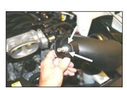
11. Install the supplied grommet (#13) and aluminum fitting (#16) into the Airaid intake tube as shown.
