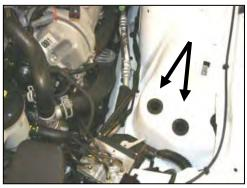
**4.** Remove the complete factory intake. Use caution to retain the factory grommets in the inner fender.
