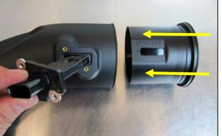
4. Install the Grommets and Fittings into the Airaid intake 5. Using the supplied Torx driver, remove the MAF sen-
