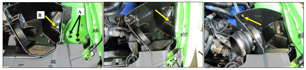
7. Transfer the factory air box mounting grommets. A) Locate and remove the Two Lower air box mounting grommets, and install them in the inner fender. B) Remove the Upper air box mounting grommet and steel sleeve, and re-install into the Airaid Cool Air Box
