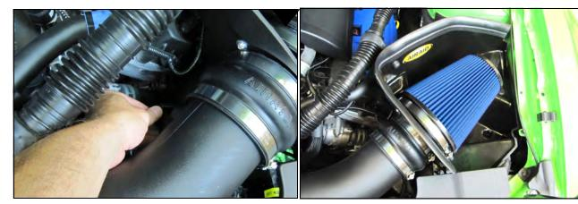
located in the lower back side of the intake. Slide the locking tab back into the connector.
