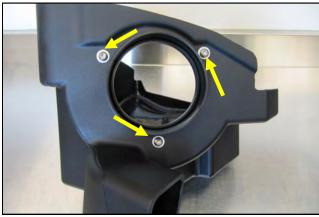
6. Install the filter adapter (#8) using three 1/4-20 button head bolts (#10), and flat washers (#11) into the Airaid Cool Air Box as shown.
