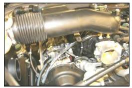
14. Remove the factory intake tube.
