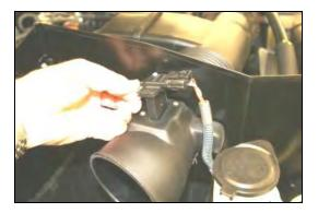
**8.** Re-route MAF wire harness under the intake tube, and around the front of the airbox. Install MAF sensor into the MAF adapter , using two supplied button head screws (#19). **DO NOT USE FACTORY SCREWS!**
