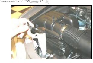
**2.** Loosen hose clamp where intake tube connects to the airbox.
