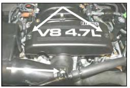
**13.** Remove two 10mm nuts, and the beauty cover from the top of the engine. Remove one bolt thru the Adel clamp that holds the air conditioning hose to the intake tube. Loosen hose clamps on each end of the factory intake tube.
