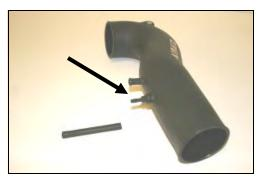
**16.** Install the barbed fitting (#11) into the MIT as shown, and then slide the 1/4"x4" hose (#13) over the fitting.
