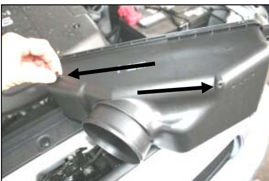
8. Install the two rubber washers (#19) onto the two plastic plugs (#18) that are provided in the hardware kit, and insert them into the two weep holes in the factory air cleaner cover removed in step #4, as shown
