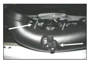
10. Install the 1/8" barbed fitting (#20) into the Airaid intake tube (#2) as shown. Next install the MAF sensor removed in step #9, into the Airaid intake tube and secure it with two 8/32" x 3/8" (#12) button head screws. Do Not Use The Factory Screws!
