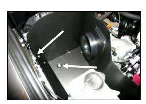
**8.** Install the **CAD** assembly into the vehicle. Align the hole in the bottom over the captured nut in the fender well. Install one 6mm hex bolt (#16), and washer (#14). Leave loose for now. Next reinstall the factory bolt removed in step #6, thru the bracket, into the ground anchor in the fender well. This bolt can be tightened now.
