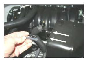
**4.** Disconnect the breather hose from the back of the factory intake tube and the valve cover. Disconnect the 1/8" vacuum hose from the back of the factory intake tube and the vacuum connection on the engine. These hoses will be replaced with Airaid hoses later in the install.
