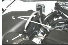
**3. A.**) Squeeze the tab on the Mass Air Flow (MAF) sensor wiring connector and disconnect it from the sensor. **B.**) Squeeze the tabs on the bottom of the two wiring harness anchors, and remove them from their respective anchor points.
