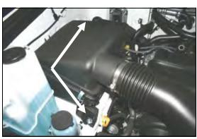
**5.** Using a 10mm socket, loosen the two bolts that anchor the factory airbox to the inner fenderwell. One is on the front of the airbox, and the other is on the rear. Pull the factory intake tube away from the throttle body and remove the complete factory intake assembly from the vehicle.
