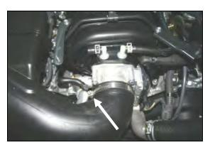
**2.** Using a 10mm socket, loosen the hose clamp that secures the factory intake tube to the throttle body.
