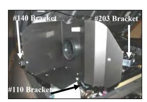
7. Assemble the Cool Air Dam panels (#3 & #4) as shown using four 6-32 screws (#9), washers (#10), and keps nuts (#11). Install the filter adapter (#5) using three 1/4" button head bolts (#13) and washers (#14). Install the 3 brackets (#24), (#25), and (#26) as shown using three 1/4" bolts (#13), washers (#14), and nuts (#15). Just snug the bolts for now, they will be adjusted later.
