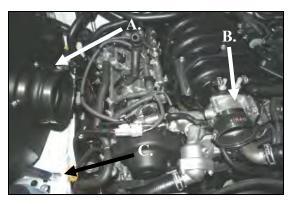
11. A) Install the hump hose (#7) onto the filter adapter using two #72 hose clamps (#19). B) Install the smaller end of the reducer coupler (#6) onto the throttle body using one #52 hose clamp (#17). Next install the #56 hose clamp (#18) over the coupler and leave it loose. C) Now align the #110 bracket (#24) over the captured nut in the fender well and install one 6mm bolt (#16) and washer (#14). Leave loose until final adjustment.
