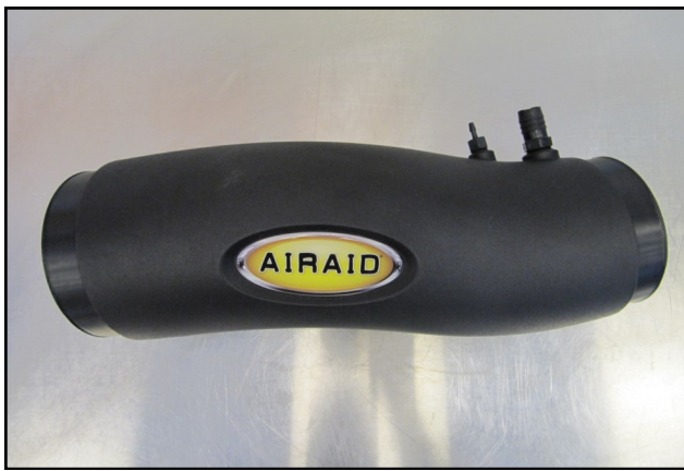
9. Install the 1/8" and 3/8" barbed fittings (#s 11 and 12) into the Airaid Intake Tube as shown.
