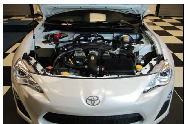
Double check your work ! Make sure there is no foreign material in the intake path. Make sure all clamps, hoses, bolts, and screws are tight. Double check the hood clearance!
