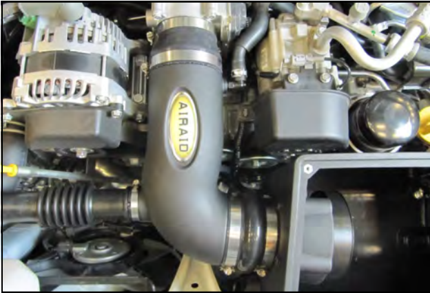
13. Install the Intake Tube and tighten all of the clamps. Connect the crank case breather to the Barbed Fitting and secure it using the OEM spring clamp. Insert the resonator into the Intake Tube and tighten the clamp.
