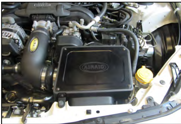
16. Install the Air Box Lid using the 10-24 Button Head Screws and the #10 Washers.
