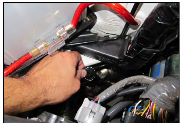
18. Place the Firewall Grommet into the bulkhead. NOTE: The resonator Delete option has no positive or negative effect on performance
