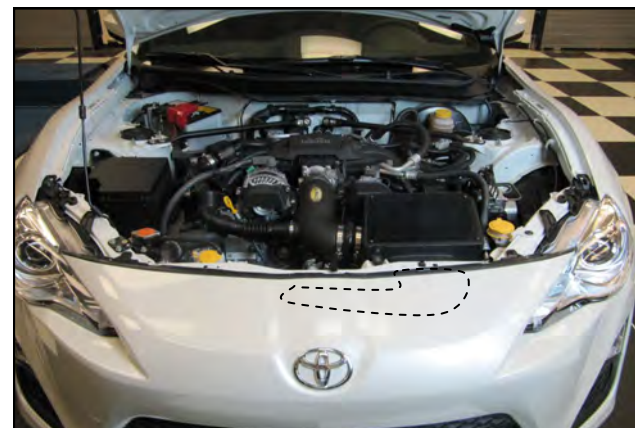
20. With help from an assistant. The inlet can be removed without removing the entire bumper cover. Simply remove all of the topside fasteners and pull back on the cover. Have an assistant remove the two 6mm bolts in the tube and remove.
