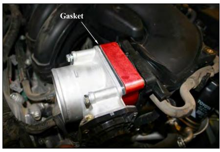
**6.** Slide the Poweraid Spacer (#1) and gasket (#2) between the intake manifold and the throttlebody. Make sure the "Flow" arrow on the spacer is pointing towards the intake manifold, and the gasket is next to the throttlebody. Install the 4 supplied 6mm x 75mm bolts (#3) and flat washers (#4) thru the throttlebody, gasket, spacer, into the intake manifold and tighten evenly to the vehicle manufacturer's specifications.
