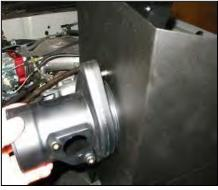
7. Using two supplied 1/4-20 bolts and washers, mount the Airaid filter adapter to the Airaid Cool Air Dam.
