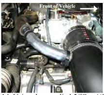
14. Using the supplied 5/8" to ½" barbed connector and ½" x 4" breather hose, connect the factory hose located by the throttle body to the Airaid intake tube. Use two supplied #16 Speed clamps to secure the hose to the barbed ends.
