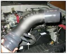
9. Install two supplied ½" NPT barbed fittings in Airaid intake tube. (Note: Install 3/8" fitting in the forward hole and the ¼" fitting in the back hole) Slide hump hose and two #52 hose clamps on large end of intake tube and slide coupler with two #48 hose clamps on small end of tube. (Note: leave all hose clamps loose for final assembly)
