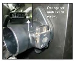
8. Using the two 8-32 Allen head screws and two plastic spacers provided, mount the factory Mass Air Sensor to the Airaid filter adapter tube. (*Note: the plastic spacers are placed between the Mass Air Sensor and the Filter Adapter Tube with the screws sliding through the spacers*).
