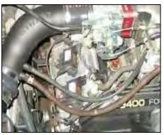
13. Connect factory 3/8" vacuum line to nylon fitting on intake tube & connect steel tube on intake manifold to ½" fitting on intake tube with ½" vacuum line provided.
