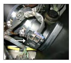
**12.** Reinstall the electrical connector to the Mass Air Sensor.
