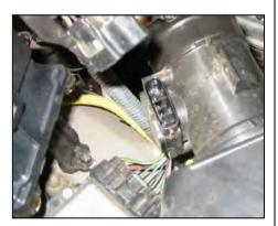
**3.** Disconnect the electrical connector from the Mass Air Sensor.
