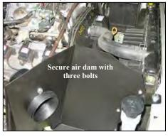
10. Position the Airaid intake assembly in place of the original, factory assembly. Using three supplied 8mm bolts and washers, mount the Airaid assembly using the three original/factory mounting points.
