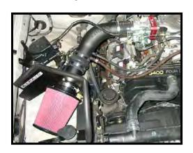
Syndhellell Do Not Oil Synthamax Air Filters <u>do not</u> require <u>oil</u>. Service air filter as needed by cleaning with common non-petroleum all-purpose household cleaner and water. Simple Green®, Formula 409® or equivalent works great. Apply cleanerif necessary. Do not apply high pressure water or air to clean filter. Allow filter to air dry and reinstall to outside of air filter and allow to soak. Then flush filter clean from the inside out with a garden hose and repeat steps
