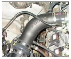
11. Connect the Airaid intake tube to the engine by sliding the coupler over the throttle body & adjust the intake tube to insure proper alignment from the throttle body to the air filter adapter. (Note: Leave a gap between the tube and the air filter adapter to allow for engine movement)
