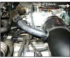
14. Using supplied 5/8" to ½" barbed connector and ½" x 4" hose; connect the factory hose located by the throttle body to the Airaid intake tube. Use two supplied #16 Speed clamps to secure the hose to the barbed ends.
