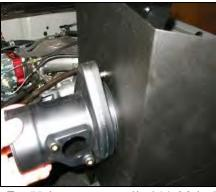
7. Using two supplied ¼-20 bolts and washers, mount the Airaid filter adapter to the Airaid Cool Air Dam.
