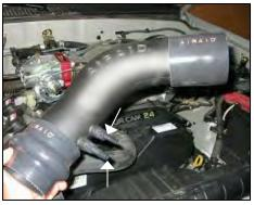
9. Install two supplied ¼" barbed fittings in Airaid intake tube. (Note: Install 3/8" fitting in the forward hole and the ¼" fitting in the back hole) Slide hump hose and two #52 hose clamps on large end of intake tube and slide coupler with two #48 hose clamps on small end of tube. (Note: leave all hose clamps loose for final assembly)
