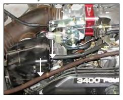
2. Remove factory vacuum line or lines from the factory air box and intake tube. (*Note: Retain the 3/8" vacuum hose*)
