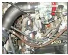
13. Connect factory 3/8" vacuum line to nylon fitting on intake tube & connect steel tube on intake manifold to ½" fitting on intake tube with ¼" vacuum line provided.
