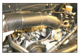
12. Remove the factory intake tube.
