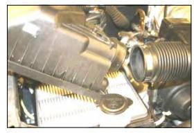
2. Unlatch the 4 clips on the factory airbox, and remove the lid. Remove the factory air filter.
