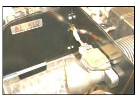
7. Install the MAF sensor into the MAF adapter (#4) and tighten down using two supplied button head bolts (#19). Do Not Use The Factory **Screws!**
