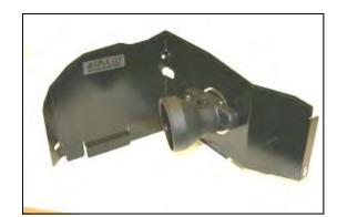
**3.** Assemble the Cool **A**ir **D**am (#2) & (#3) as shown using three screws (#14), washers (#15), and nuts (#16). Install the MAF adapter using two button head bolts (#17), and washers (#18), as shown.
