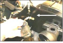
**6.** Remove the top screw on the CAD. Spread the panels slightly, and slip the wire harness thru the gap into the access hole, as shown. Reinstall the screw and tighten.
