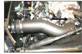
**15.** Install the Airaid **MIT** (#5) into the hump hose first, and then into the coupler. Adjust the MIT snugly against the throttle body and tighten the all four clamps. Install the supplied button head bolt (#17), and washer (#18) thru the Adel clamp, and thread into the MIT. (See arrow)
