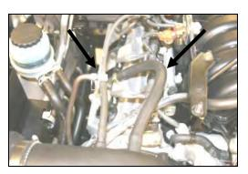
**18.** Install the vacuum tee (#12) into the 1/4"x4" hose (#13), and reconnect the factory 1/4" and 1/8" vacuum lines to the tee as shown. Install the 1/2"x13" breather hose (#8) onto the valve cover and to the MIT as shown.
