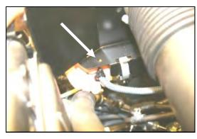
**9.** Slip hose mount (#20) over MAF wire harness, and into hole in bottom of CAD. This will keep the harness from chafing.
