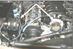
15. Install the hump hose (#7) on the MAF adapter (#4) with two hose clamps (#10). Install the reducer (#6), small end first, onto the throttle body with two hose clamps (#10). Leave the clamps loose for now.
