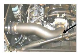
17. Install the MIT (#5) into the hump hose (#7), and then into the reducer (#6). Adjust the MIT snugly against the throttle body, and tighten all 4 hose clamps. Install the supplied button head bolt (#17), and washer (#18), thru the Adel clamp and into the MIT to hold the air conditioning hose.
