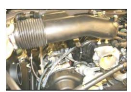
14. Remove the factory intake tube.
