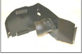
**6.** Assemble Cool Air **D**am (#2) & (#3) using three screws (#14), washers (#15), and nuts (#16). Install MAF adapter (#4) using two button head bolts (#17), and washers (#18), as shown.
