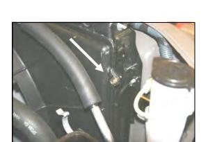
2. Loosen hose clamp where intake tube connects
