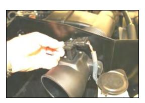
**8.** Re-route MAF wire harness under the intake tube, and around the front of the airbox. Install MAF sensor into the MAF adapter, using two supplied button head screws (#19). **DO NOT USE FACTORY SCREWS!**
