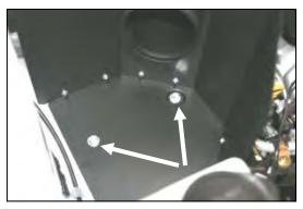
**12.** Install the CAD into the vehicle by aligning the hump hose with the tube on the factory airbox, and then aligning the two holes in the bottom of the CAD with the two mounting holes on the inner fender. Install the two supplied 8mm bolts (#14) and washers (#15).
