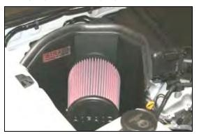
**15.** Install the Airaid Premium Filter (#1) on the CAD tube and tighten the clamp. Next install the weather strip (#7) on top of the CAD as shown. For an easier install, start at the fender side of the CAD and work your way towards the radiator.
