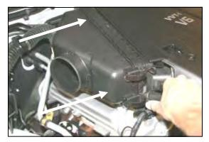
**9.** Re-install the factory airbox cover, and re-latch both clips.
