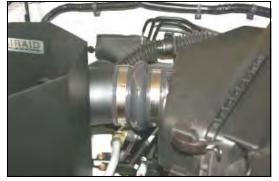
**14.** Center the hump hose between the tube on the factory airbox, and the tube on the CAD, adjust for fit, and tighten the hose clamps.
