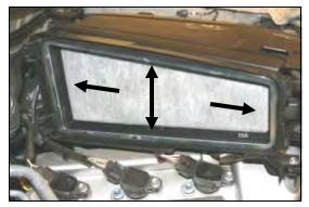
**7.** Re-install the gasket assembly back into the factory airbox as shown. Do not tamper with the factory hydrocarbon filter as this will void the vehicle manufacturer's warranty, and street legal status in the state of California.
