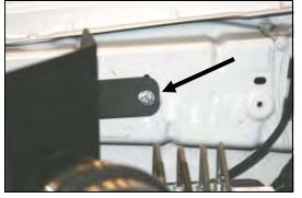
**13.** Install the supplied 6mm bolt (#12) and washer (#13) thru the tab on the CAD and into the threaded hole in the side of the fender.
