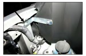
13. Fasten the #203 bracket (#26) to the existing hole in the radiator support using one 1/4-20x1/2" button head bolt (#13) washer (#14), and serrated nut (#15). Tighten all nuts and bolts that hold the CAD to the vehicle at this time.
