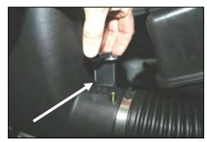
**9.** Remove two Phillips head screws and remove the **MAF** sensor from the factory intake tube. It will be reinstalled in step #10.
