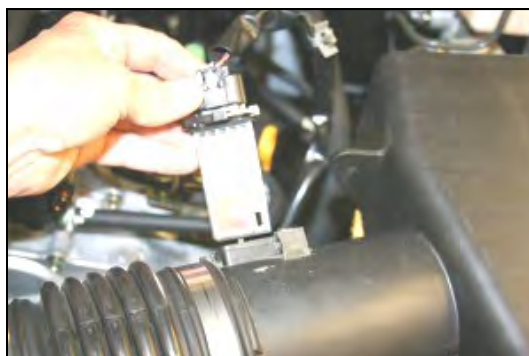
5. Without disconnecting the MAF sensor, remove it from the factory airbox lid, and set it aside. It is important to note the direction of the MAF sensor when removed, as to assure correct reinstallation later in the install process. The MAF sensor must be installed in the correct direction for proper air flow calibration.
