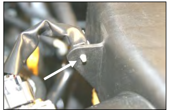
3. Using pliers, carefully squeeze the two tabs together, and remove the wire loom retainer from the factory airbox lid.
