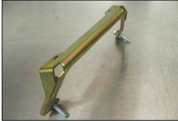
14. Remove the factory engine cover mounting bracket from the intake manifold and install the two 6mm x30mm Bolts (#10) as shown. They are to be installed from behind and protrude forward when installed properly.
