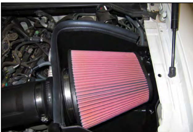
16. Install the Airaid Premium Filter (#1) onto the Filter Adapter then install the Weather Strip (#7) onto the top of the Cold Air Box with the contour rolling away from the Filter.
