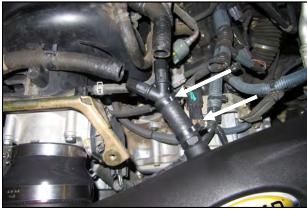
11. Install the 5/8" Hose (#16) onto the Barbed fitting in the Intake Tube. Insert the Barbed "Y" Fitting (#14) into the 5/8" Hose and secure using the two Speed Clamps (#17).
