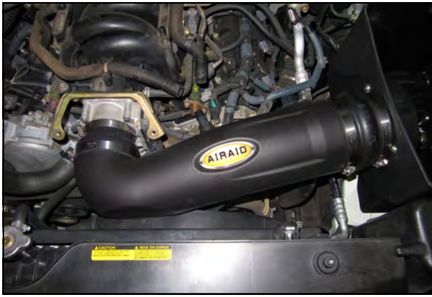
10. Install the Airaid Intake Tube into the Hump Hose first, and then into the Reducing Coupler. Adjust for fit, and tighten all four Hose Clamps.
