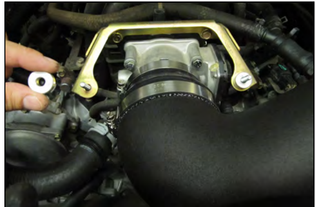
15. Reinstall the bracket onto the intake manifold and place a Spacer (#13) onto each 6mm bolt.
