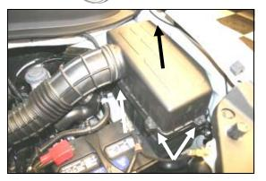
1. <u>Disconnect negative battery cable.</u> Loosen the 4 factory screws that hold the factory air cleaner lid to the air cleaner base.
