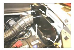
**5.** Install the Quick Fit Panel (#2) onto the top of the factory air cleaner base. Align the 4 holes, install and tighten the 4 supplied 5mm screws (#4). Carefully slide the factory intake tube onto the Quick Fit Panel Tube. Make sure it is installed at least one inch onto the tube as shown.
