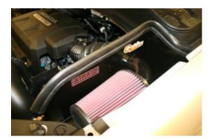
**7.** Install the supplied weather strip (#3) onto the top of the Quick Fit Panel, starting at the left fender, and working your way towards the front of the vehicle.
