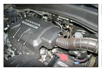
1. <u>Disconnect the negative battery cable!</u> Using a flat blade screwdriver, turn the three plastic keepers at the front of the engine beauty cover. Remove the engine beauty cover by lifting up and releasing it from the grommets.
