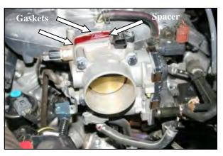
4. Install the spacer (#1) (with the flat side of the helix bore facing the throttlebody) between the intake manifold, and the throttlebody with one of the supplied gaskets (#2) on each side of the spacer. Insert four 8mm x 75mm Hex Bolts (#3), and 8mm Flat Washers (#4) through the throttlebody, Poweraid Spacer, and into the intake manifold. Using a 13mm socket, tighten all 4 throttle body bolts evenly, to the manufacturer's specifications.
