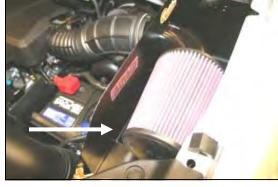
**6.** Install the Airaid Premium Filter (#1) onto the Quick Fit Panel Tube as shown, and tighten the clamp.
