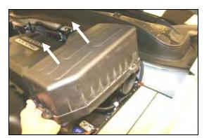
**3.** Remove the factory air cleaner lid from the vehicle.
