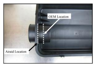
1. Notice the two stops on the mounting tube inside the air box. The first is the stop location for the OEM filter. The second stop, at the wall of the air box, is to be the Airaid stop.
