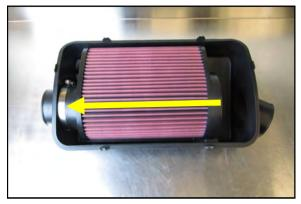
2. Install the Airaid filter into the RZR air box as shown, with the mounting flange all the way onto the mounting tube. Tighten the clamp. and reinstall the air box lid.
