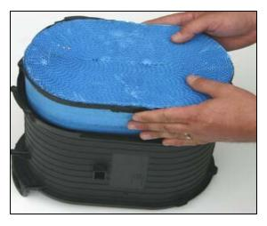
**3.** Remove the element from the filter housing and discard the element. Remove all remaining glue from the inside surface of the housing and clean surface using a rag.
