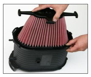
**4.** Insert the Airaid Premium Filter into the factory housing. The filter must be fully inserted into the bottom of the housing. Install the factory filter housing with the Airaid Premium Filter in the reverse order. Double check your work to insure that all connections are tight there are no foreign objects in the intake system.
