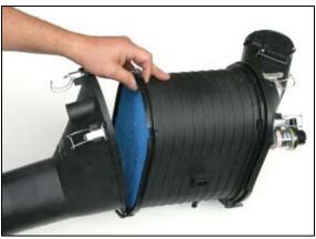
1. Remove the factory filter housing from the intake assembly by separating the inlet and outlet as shown above. Note: This step is performed in the vehicle. The vehicle is not shown in the pictures for added clarity.
