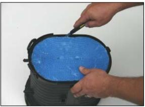
**2.** The air filter element is bonded to the housing on inlet side. Using a utility knife, carefully separate the filter element from the air filter housing as shown above. The utility knife will cut easily through the black glue that is used to bond the element to the housing. Use extra care to avoid personal injury from the sharp tool.
