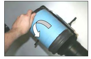
**2.** Remove the factory air filter by gently prying it towards the passenger side of the airbox, and then lifting it straight up.
