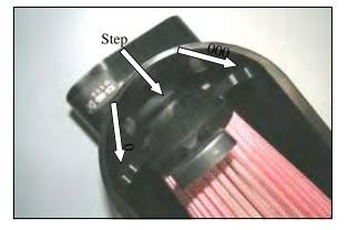
**5.** Locate the "step" on the bottom of the factory airbox. Make sure that the tab on the air filter is aligned with it. Next, align the two side tabs on the air filter with the side of the factory airbox.
