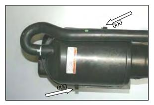
**6.** Reinstall the factory airbox lid and re-latch the two factory clips.
