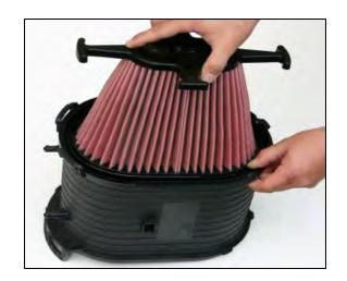
4. Insert the Airaid Premium Filter into the factory housing. The filter must be fully inserted into the bottom of the housing. Install the factory filter using with the Airaid Premium Filter in the reverse order. Double check your work to insure that all connections are tight there are no foreign objects in the intake system.
