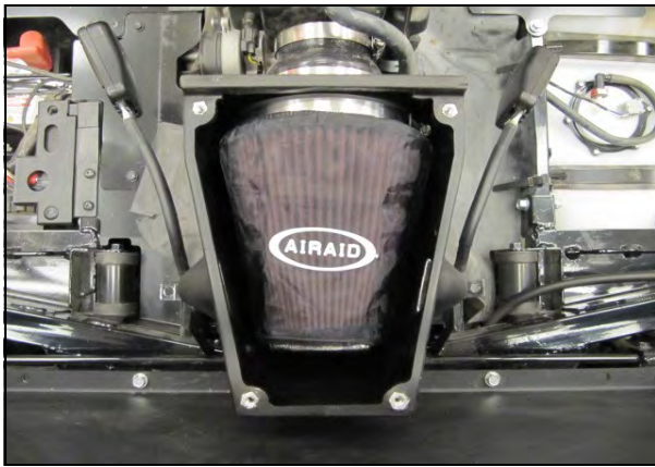
13. Slip the Pre-Filter (#15) over the Airaid Premium Filter.
