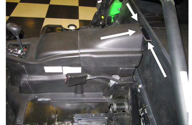
14. Reinstall the factory covers in the reverse order of removal. Reconnect the battery terminal and reinstall the seats. Notice that the Air inlet is now located outside of the engine cover.
