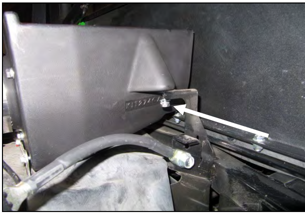
11. Secure the rear half of the CAB assembly to the Horizontal brackets using two 1/4-20 x 5/8" bolts (#6), 1/4" lock washers, and 1/4" Flat washers.
