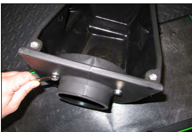
7. Install the Filter Adapter on the Cold Air Box, or CAB (#2) as shown using three 1/4-20 x 5/8" Bolts (#6), 1/4" lock washers (#10), and 1/4" Flat washers (#9). Do not over tighten.
