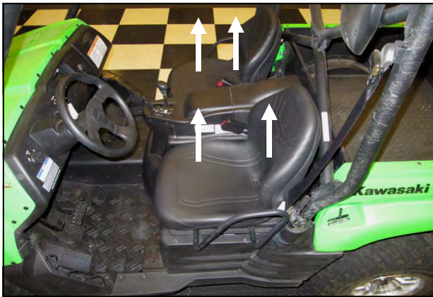
1. Remove both the driver and the passenger side seats. Disconnect the negative side battery terminal.
