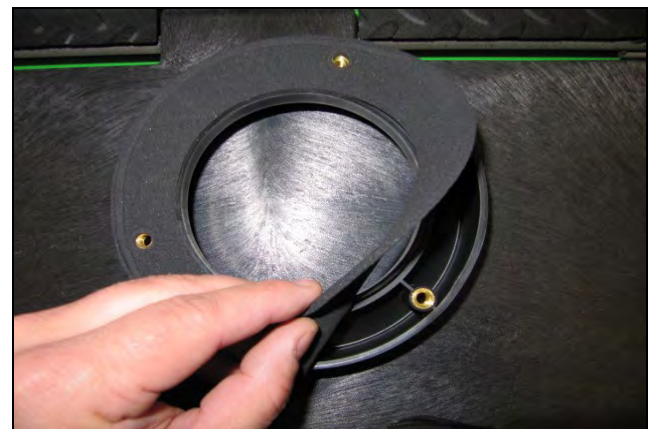
6. Prepare the Filter Adapter (#4) for installation by attaching the gasket (#13) and lining up the bolt holes.
