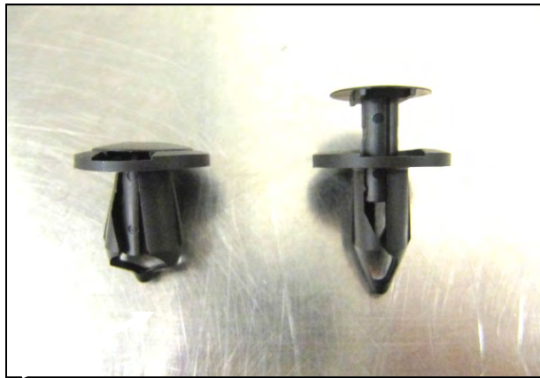
2. The engine covers needing to be removed for this installation are primarily held in place with the use of nylon rivets. Nylon rivets are reusable if care is taken during their removal and installation. Using a small standard blade screwdriver, gently pry up on the center post until the entire rivet can be pulled freely from the panel. Rivet installation is the opposite.
