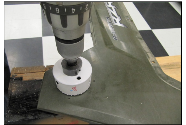
32. Cut the large hole in the panel using a drill with a 3" hole saw.
