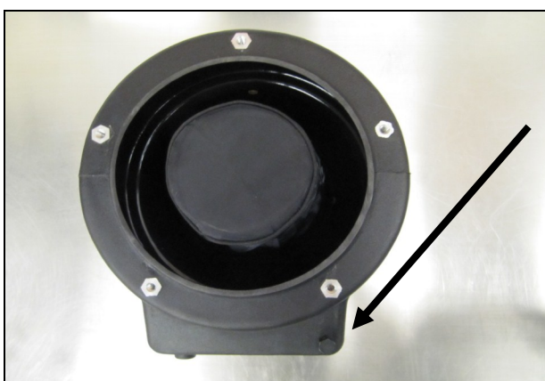
22. Install the 1/8" NPT Drain Plug (#25) into the Airaid Air Box.
