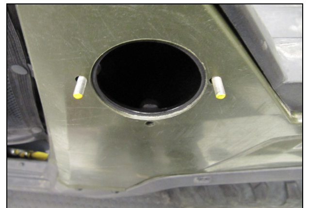
44 Temporarily install two Threaded Studs (#11), finger tight, into the Riser Tube as shown.
