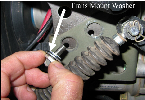
27. Fasten the Transmission Bracket to the transmission using the two 1/4-20 x 5/8" Hex Head Bolts (#12), 1/4-20 Flat Washers—Large (#16), Trans Mount Washers (#10), and 1/4-20 Lock Nuts (#17).
