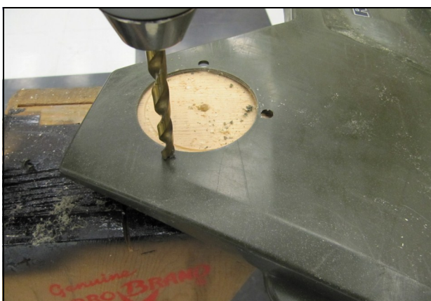
33. Drill 5/16" bolt holes in the Panel.
