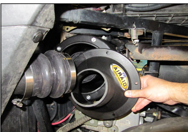
1. Loosen the Clamps on the Hump Hose and slide it back. Remove the 1/4" bolts and washers from the Air-Box Top and slide out the Top
