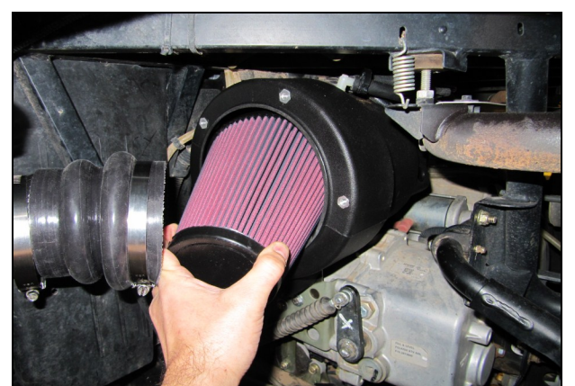
3. . The Filter can now be removed for service and inspection. Thoroughly inspect the interior of the Air Box for water and large pieces of debris that may have been ingested.
