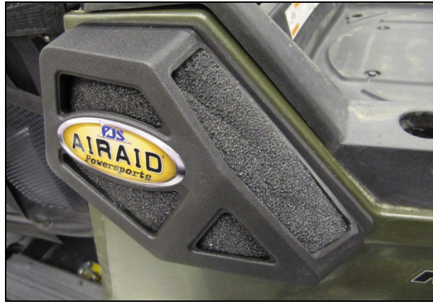
40. Insert the Foam Pre Filter (#6) into the Air Scoop as shown.
