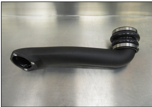
34. Slide the Hump Hose (#8) and clamps onto the Riser Tube (#4) as shown. The #52 Clamp (#19) is to be installed on the Tube side and the #60 Clamp (#20) on the other. Leave the clamps loose for now.
