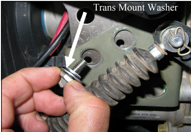
27. Fasten the Transmission Bracket to the transmission using the two 1/4-20 x 5/8" Hex Head Bolts (#12), 1/4-20 Flat Washers—Large (#16), Trans Mount Washers (#10), and 1/4-20 Lock Nuts (#17). Note: It is intended for the Trans Mount Washers to fit inside the holes in the OEM bracket when properly installed.
