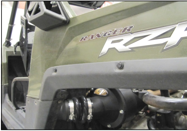
39. Re install the panel, Scoop, and Riser Tube onto the vehicle. Slide the Hump Hose and clamps onto the Air Box Inlet, and tighten the Clamps.
