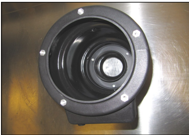
18. Mount the Filter Adapter and gasket inside the Airaid Cold Air Box (#2) using three 1/4-20 x 5/8" Hex Bolts (#12), 1/4" Flat Washers (#14), and 1/4" Nylock Nuts (#17).
