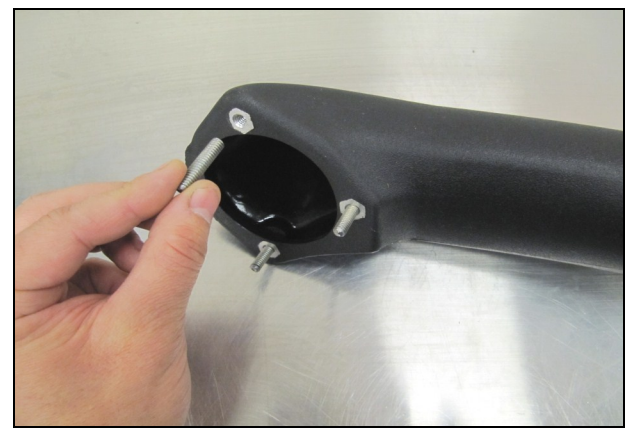
35. Install the Threaded Studs (#11) into the Riser Tube.
