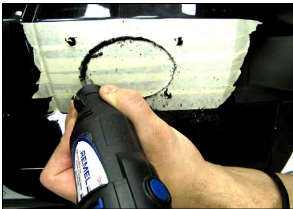
13. Using a Dremel type rotary tool and a 1/8" drill bit, plunge into the inner oval at medium speed and cut along the line until the center falls out. Remove the tape.
