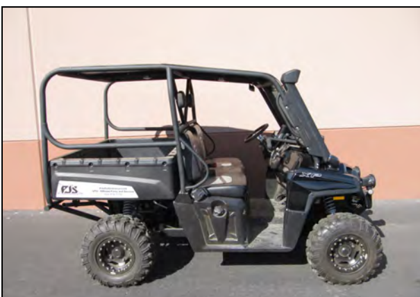
22. Double check your work! Make sure there is no foreign material in the intake path. Make sure all clamps, hoses, bolts, and screws are tight. Make sure all clamps, hoses, bolts, and screws are tight. Periodically check the tightness of all hose clamps.
