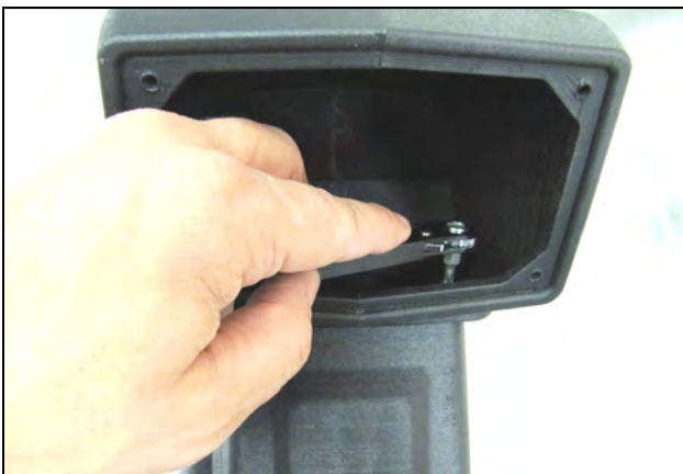
3. Mount the Snorkel Inlet to the Snorkel Tube (#2), using the four Torx screws (#14) and a 90deg. Low Profile Ratcheting Screwdriver.
