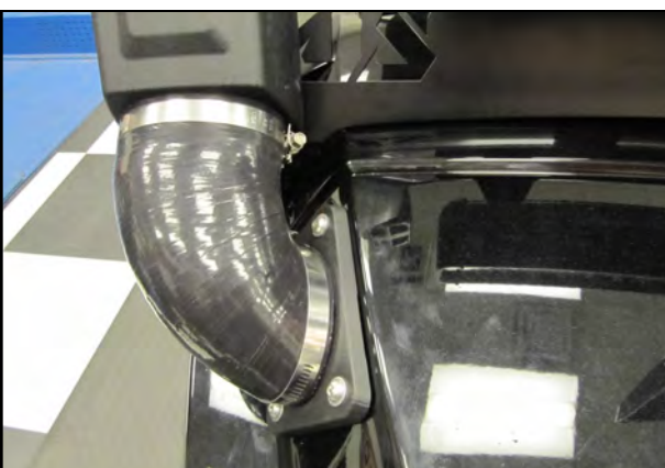
19. Install the trimmed Coupler with clamps (#9) onto the Snorkel tube and the Fender adapter. Tighten the Hose clamps and the three Snorkel Tube Clamps on the cage.
