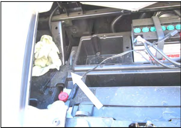
9. Place a shop towel inside of the factory inlet hose to prevent debris from entering.
