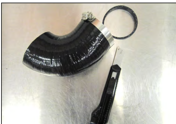
18. Once you have your coupler length marked, slide a hose clamp (#9) onto the coupler and tighten the clamp along the mark. Use the hose clamp as a guide to trim the coupler to length with a sharp utility knife.
