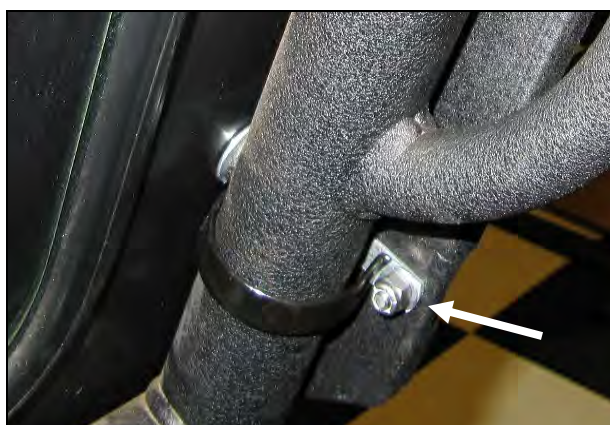
7. Attach the Snorkel Tube to the Loop Clamps using three 1/4-20 Button Head Bolts (#11), 1/4-20 Locknuts (#12), and Flat washers (#13). Leave all hardware finger tight at this time to allow for proper alignment .
