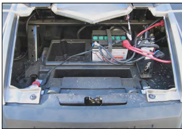
1. Lift the hood, secure it in the upright position, and disconnect the battery or batteries.
