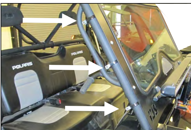
6. Preinstall the three Loop Clamps (#10) onto the right front A pillar of the cage.
