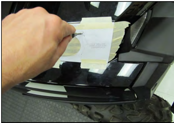
10. Prepare the right front fender for cutting by covering the entire area with masking tape. Cut out the Template and align all four edges against the radius of the fender. Tape down the template and mark the bolt holes with a center punch.
