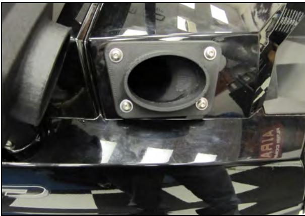
16. Mount the Adapter to the fender using Four 1/4-20 Button Head Bolts (#11), eight 1/4" Flat Washers (#13), and four 1/4-20 Locknuts (#12). Tighten the factory air inlet hose clamp.
