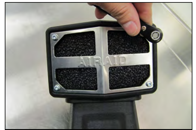
5. Install the Snorkel Screen (#4) onto the Inlet using the four 8-32 Button Head Screws(15).
