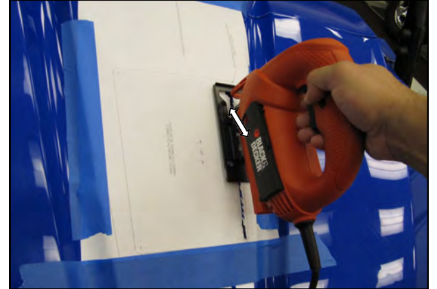
15. Using a jig saw, cut out the center section of the hood.
