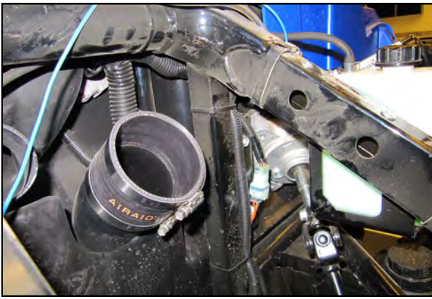
10. Install the Silicone Coupler (#8) and Two #48 Hose Clamps (#10) onto the factory intake tube. Leave the Clamps loose for now.
