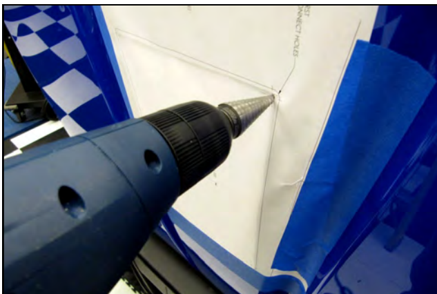
14. Using a 1/8" bit , drill out the punched holes on the hood. Finish the holes using a 1/2" bit or UniBit.
