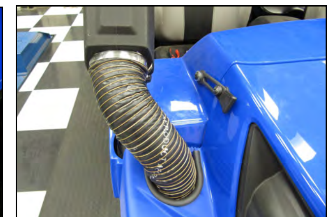
39. Align the Snorkel and Ducting and verify the opening and closing action of the hood is not adversely effected. Tighten all of the Clamp bolts when done.
