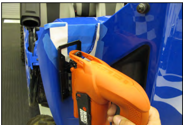
31. Using a jig saw or equivalent, follow the template and cut out the Duct relief.
