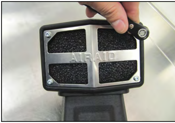
26. Install the Snorkel Screen (#14) onto the Inlet using the four 8-32 Button Head Screws(#29).
