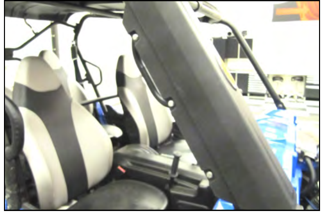
27. Attach the Snorkel Tube to the Loop Clamps using three 1/4-20 x 1 1/4 Bolts (#27), 1/4-20 Locknuts (#28), and Flat washers (#21). Leave all hardware finger tight at this time to allow for proper alignment
