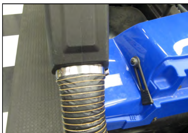
35. Install the other end of the Ducting onto the Snorkel tube using the last #48 Hose Clamp (#18).
