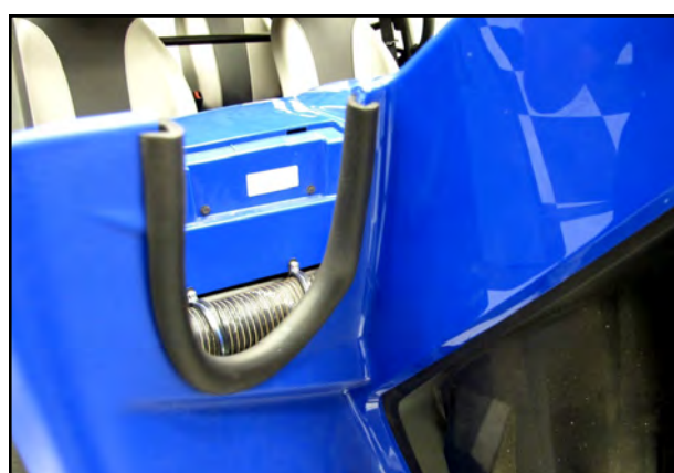
38. Slide the 10" Edge Trim (#25) over the cut out on the Hood.
