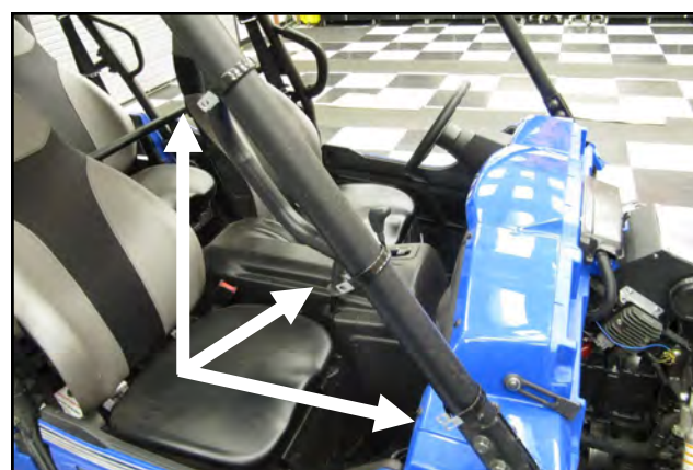
23. Side the three small Loop Clamps (#26) onto the roll cage A pillar as shown.
