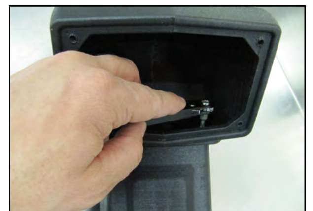
24. Mount the Snorkel Inlet(#13) to the Snorkel Tube (#12), using the four Torx screws (#33), Torx Bit #18 and a 90deg. Low Profile Ratcheting Screwdriver.
