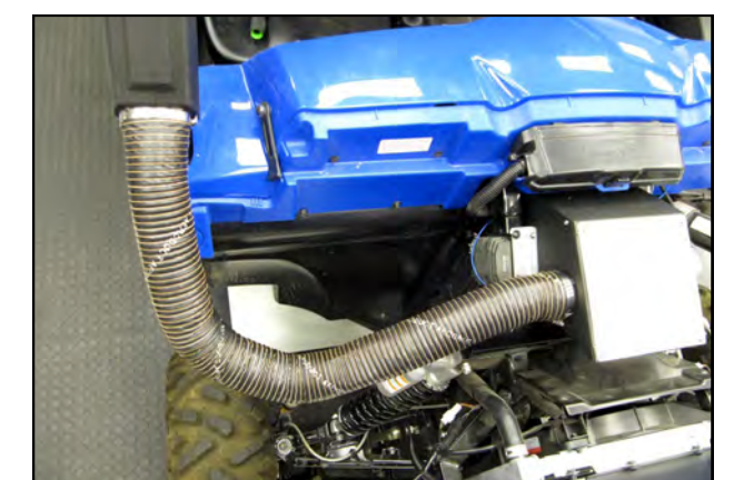
36. Full view of Duct routing.
