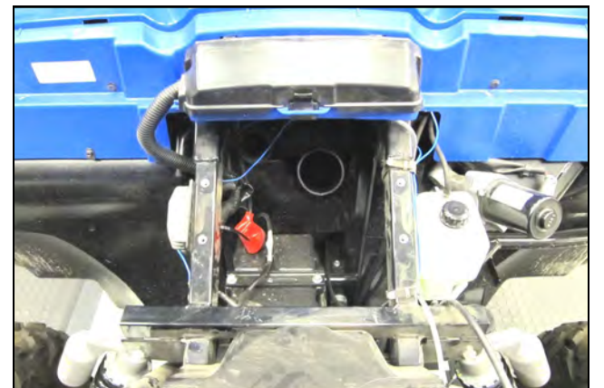
3. Remove the factory airbox and couplers from the vehicle.
