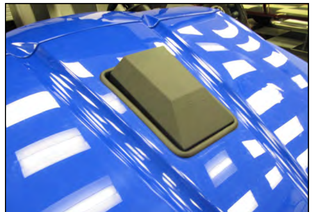
21. Lower the hood down onto the vehicle and secure it. Align the Hood Scoop from left to right inside of the cut out . Raise the hood, secure the Bolts and re connect the battery.
