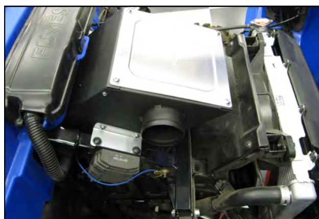
22. Install the Airbox Lid (#1) onto the Airaid performance Airbox using The four 1/4-20 x 1/2" Button Heads Bolts and 1/4" Flat Washers from the Airaid 883-306 intake.
