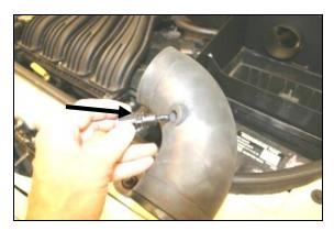
**10.** Very carefully, install the factory temperature sensor removed in step #6, into the Airaid intake tube. Make sure it is seated all the way in.
