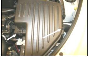
**2.** Unhook the two metal clips that hold the factory air cleaner lid to the base of the air cleaner box.
