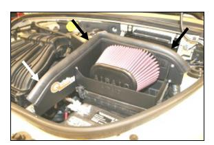
12. Install the Airaid Premium Filter (#1) onto the Quick Fit Panel, and tighten the hose clamp. Next install the weather strip (#6), as shown, onto the top of the Quick Fit Panel starting at the front and working your way towards the back.
