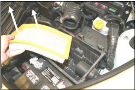
**4.** Remove the factory air filter from the base of the air cleaner box.
