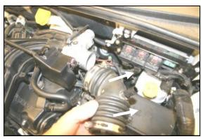
**5.** Remove the factory air intake tube from the throttle body.
