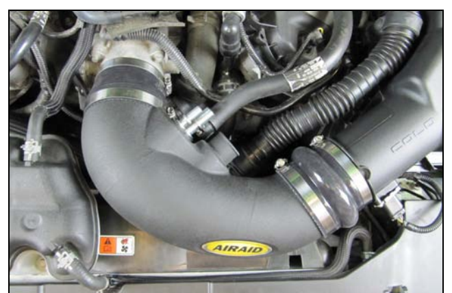
9. Insert the Intake Tube assembly into the Hump Hose first then into the Coupler on the throttle body. Align the components and tighten the Clamps.
