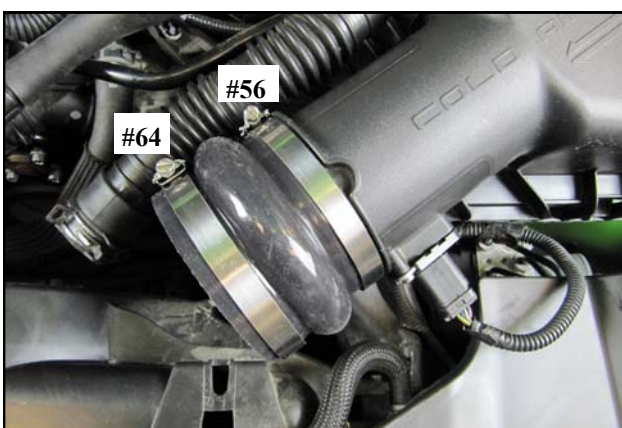
7. Slide the Hump Hose, one #56 Clamp, and one #64 Clamp onto the air box outlet as shown. Do not tighten the Clamps at this time.
