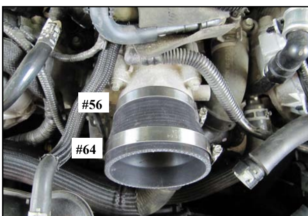
8. Install the Coupler and Clamps onto the throttle body as shown. Do not tighten the Clamps at this time.
