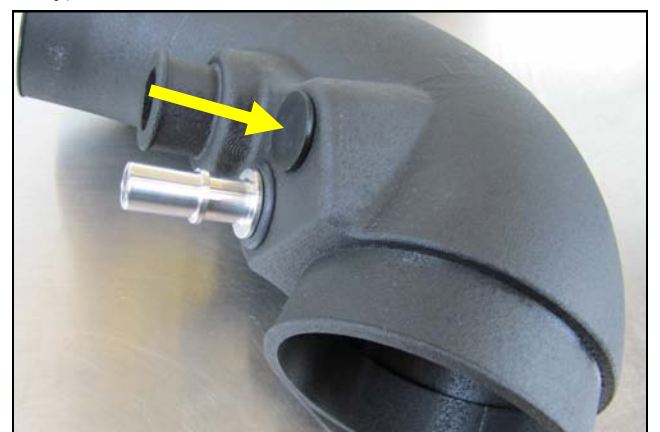
6. Manual transmission vehicles will not need the 3/8" components and will use the Blind Grommet.
