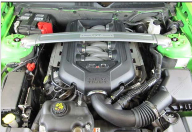
1. Disconnect the negative battery terminal. Remove the strut tower brace, if so equipped.
