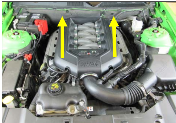
2. Lift straight up on the engine cover to unseat it from the mounting grommets and set it aside.
